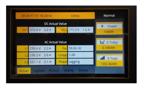
"Output Power", "Today's Generation" and "Total Generation" are shown in the right side of the display. At the bottom of the display are five most often used menus. Details are as below:
