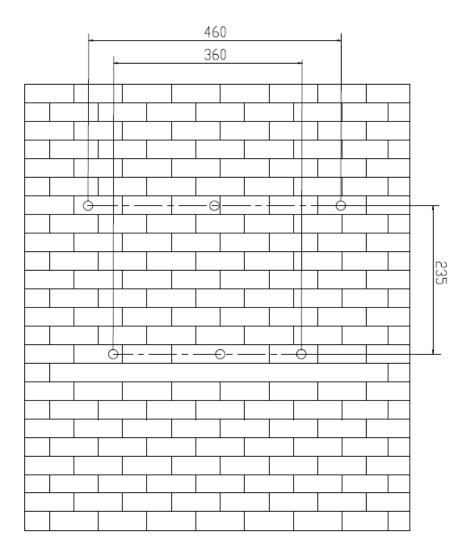
2) First, according to the marks, drill 6 holes in the wall. Then, place four expansion tubes in the holes using a rubber hammer. Next, wring 6 screws into the expansion tubes.
