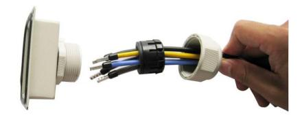
Open the plastic cover, use slot type screwdriver to press the shrapnel in the indicated position, and then put the line in the right hole, please note the sequence of the line shall in the right order: L1,L2,L3,N,PE
