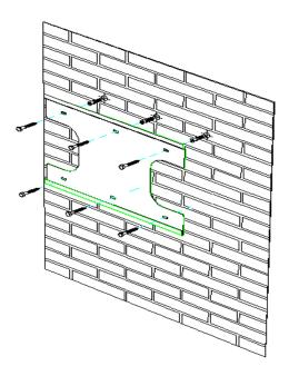
3) First check the 4 holes in the backside of the inverter. Then, lift the inverter carefully, align the 4 holes in the inverter and the 4 screws in the wall, and finally attach the inverter to the screws slightly.
